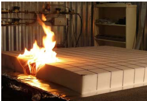
Full-scale Fire Test of Foam Specimen
