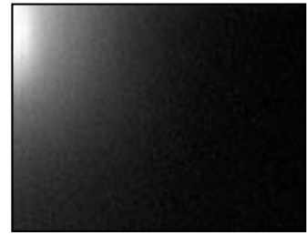
10-minute amplifier glow (electroluminescence). Older CCDs suffer from this effect which can be removed with a dark frame.
