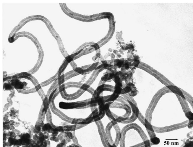
Figure 1. A typical TEM image of carbon nanotubes.
