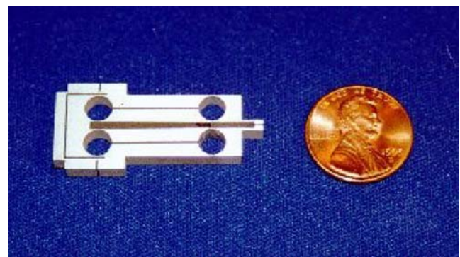
Fig. 9 Microgripper at Vanderbilt University (Goldfarb and Celanovic [16])
